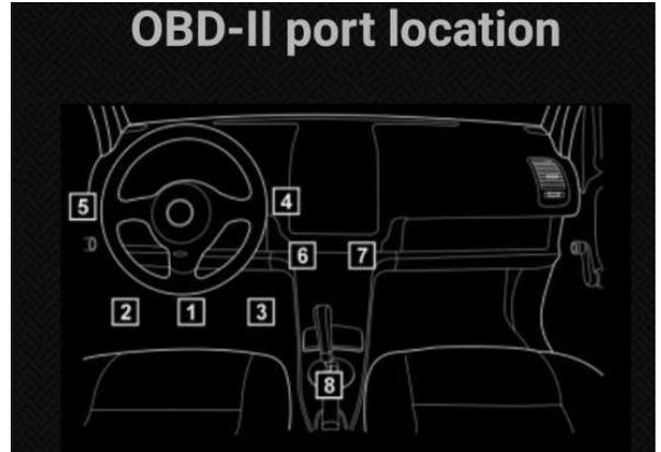
The connector may be either open or covered with an easily removable cover labelled ("OBD-II", "Diagnose," etc.). Each pin of the connector has a different purpose.
